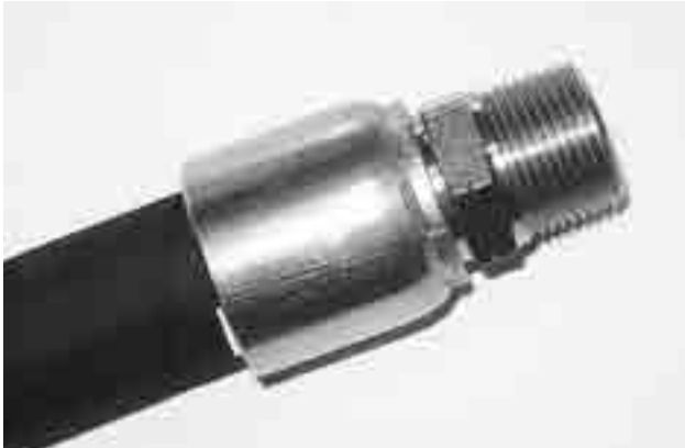
Fitting inserted on hose.
