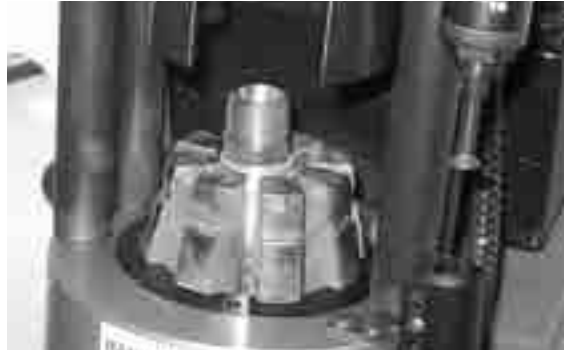
Insert hose assembly into crimper die set.
