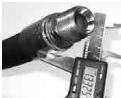
Verify crimp diameter with calipers.
